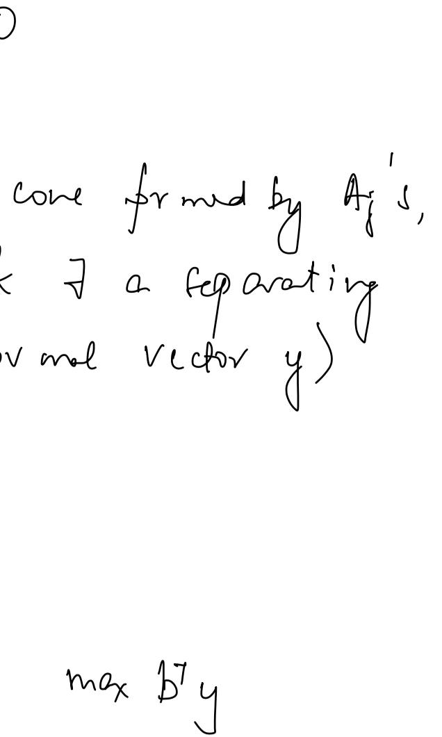
Geometric perspective: either  $b$  lies in the cone formed by  $A_j$ 's, or  $b$  lies outside &  $\exists$  a separating hyperplane (w/ normal vector  $y$ )
